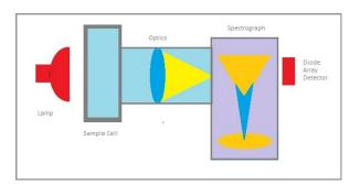
directed onto a silicon photo diode array detector. This array detector measures the intensity of the light at each frequency to produce what is called the NIT spectrum of the sample.
