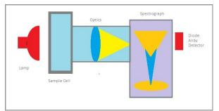
The separated light is then directed onto a silicon photo diode array detector. This array detector measures the intensity of the light at each frequency to produce what is called the NIT spectrum of the sample.
