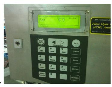
is directed onto a silicon photodiode array detector where the intensity of the light is measured at each frequency. The intensity is related to the concentration of the chemical component that absorbs at that frequency. A calibration model uses this data to compute the concentration of compounds in the sample.
