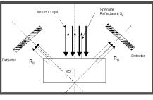
and 2500nm. The combination stretch and bend vibrations of C-H, N-H and O-H bonds lies between 1900 and 2500nm, while the first and second overtone vibrations occur between 1200 and 1800nm. The 1st and 2nd overtone regions provide good absorption spectra for transmission through liquids or reflectance off high water content solids.
