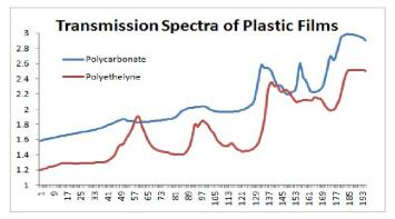
sheets, the light passes through the sample without deviation. This technique is classical transmission spectroscopy. Typically the pathlength of such samples is between 0.5 and 2mm thick.
