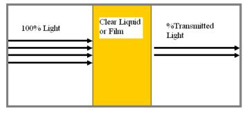
through the sample is focused onto the InGaAs detector where the electronics and software collect the interferogram. The inverse Fourier transform is applied to the interferogram to generate the NIR spectrum. For materials that are clear, i.e. Liquids, plastic films or
