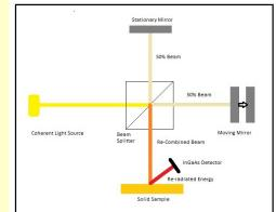
interference. The detector scans the re-combined beam over the time it takes for the mirrors to move in and out of phase. The signal collected by the detector is the interference pattern but it is called an Interferogram.
