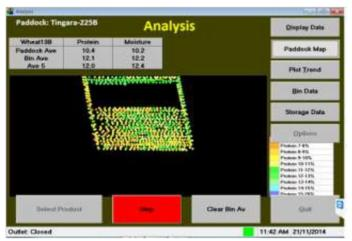
The Touch Screen PC is the control centre for the CropScan 3000H. The software displays the protein, moisture and oil data in the form of tables, trend plots, field maps and Bin Averages. The data is stored in the PC and the Bin Average data is sent to the internet where it can be viewed from a Smart Phone, tablet or PC.
