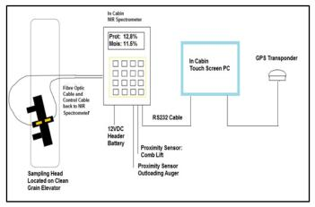
The Remote Sampling Head is mounted to the clean grain elevator. The NIR spectrometer and Touch Screen PC are located inside the cabin. The GPS receiver fitted to the combine is connected by a RS232 cable to the Touch Screen PC. A proximity sensor is located on the out loading auger and connected to the NIR spectrometer so that the system knows when the bin is being out loaded.
