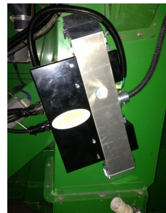
Figure 3. CropScan 3000H Sampling Head mounted on the clean grain elevator.
