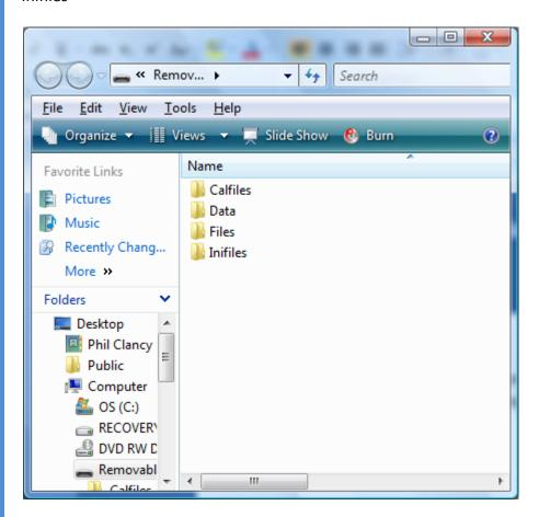
WGA Version 5.041V.26LG 15/10/10 software recognises these four new folders, named "CalFiles", "Data", "INIFiles" and "Files". The instrument will only detect data stored in these folders, anything on the root directory or any new folders created will be ignored. When files are uploaded or downloaded they will be saved or retrieved from these files.
