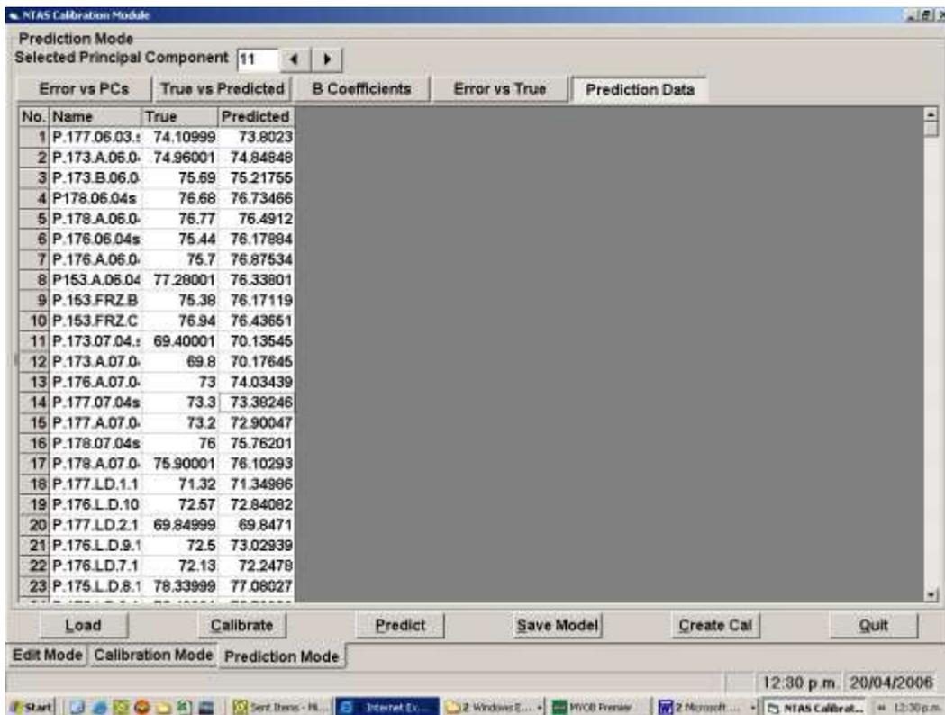
Figure 3: True versus predicted values for moisture
